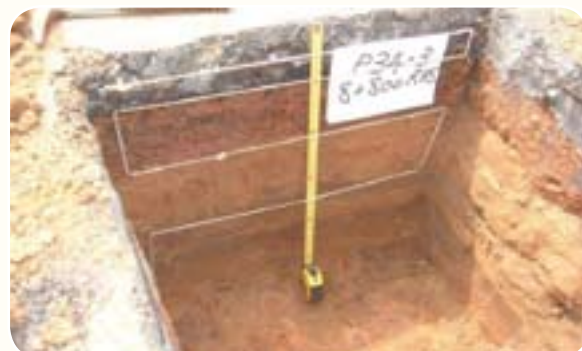
Composition of layer works on road MR34/3
