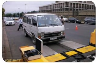
Vehicle being driven on to brake testing machine for inspection
