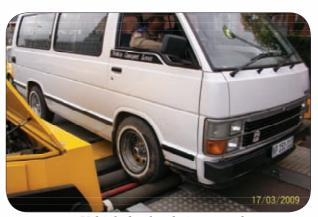
Vehicle brakes being tested
