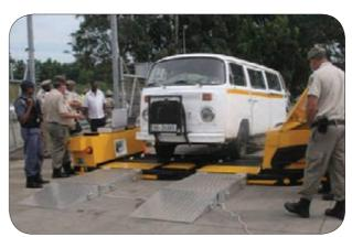
Mobile brake roller tester during the road block
