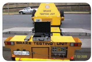
Brake testing machine set up for use
