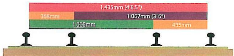
Diagram showing how four of the rail gauges used in different countries on the African continent can be arranged to use the same route by laying four rails on the same set of sleepers. By this means the expense of changing the gauge of a railway and its rolling stock is avoided.
