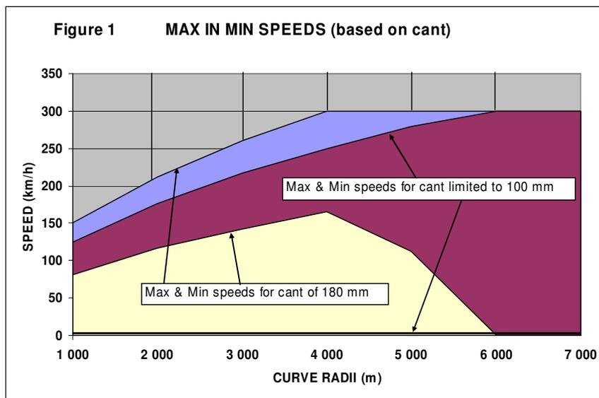
Figure 1 indicates the maximum and minimum speeds around curves for different cant conditions. The UIC task team on high speed lines recommended a maximum cant of 180
