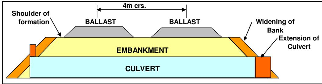
Another alternative would be to do the extension on one side only. The centre lines of the tracks would then have to be moved. Such extensions could then be done with heavy earthmoving equipment to a minimum width of approximately 2.5 meters. Fairly substantial benching could then be done into the existing embankments without endangering the tracks on the embankments. This method would however also require moving of the electrification masts and other structures.
