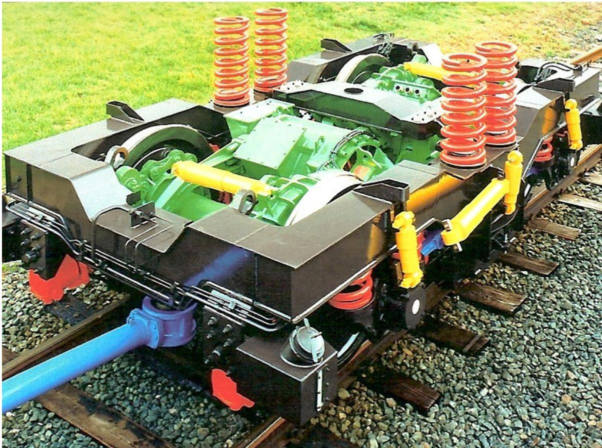
**Figure 1: A motored bogie<sup>5</sup>**
